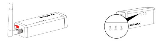
Use an Ethernet cable to connect the gateway to your wireless router or access point. The green power LED and orange Internet LED will display on to indicate successful cloud and Internet connections.
