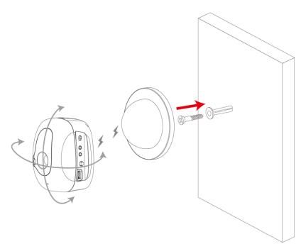
The camera unit's rear mounting hole below the magnet also allows you to mount the camera to a third party stand if you prefer.
