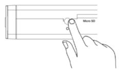
Within 30 seconds, push the Pair button on the camera unit for 2 seconds. After a few seconds, the camera's Status LED will flash quickly orange to indicate successful pairing.
