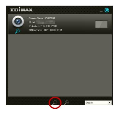
The network camera's IP address is displayed on this screen. After setup, you can enter this IP address into the URL bar of a web browser on the same local network to access your network camera's web-based configuration interface.
