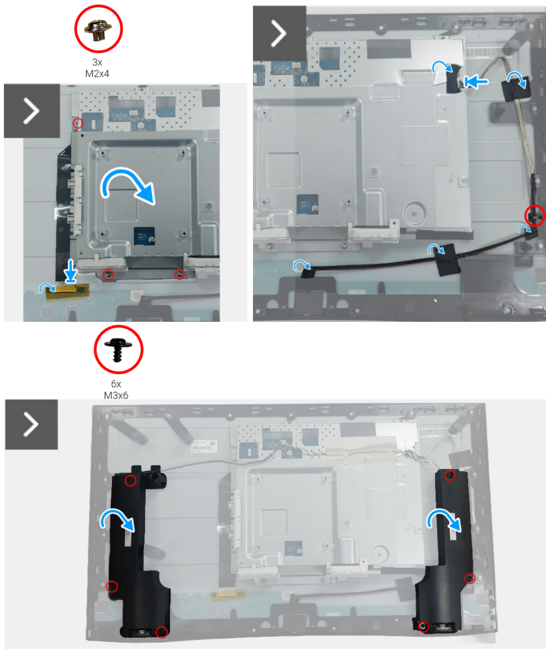
Figure 17. Installing the interface board assembly
