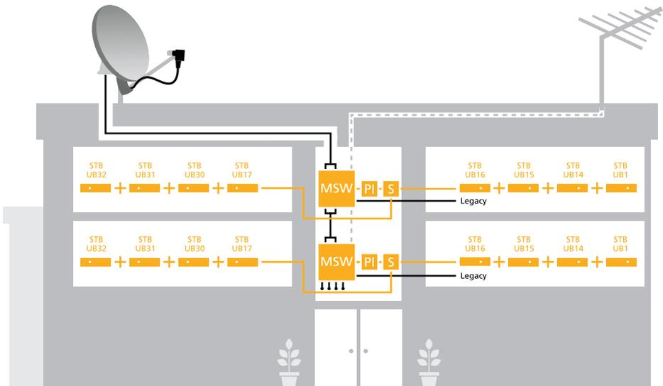
Connect the cables from the Quattro LNB to the input connectors marked with LNB V/L, V/H, H/L and H/H inputs (pay attention to identification of the Quattro LNB connectors). The multiswitch is equipped with Terrestrial input. Connect the Terrestrial antenna to this input:
