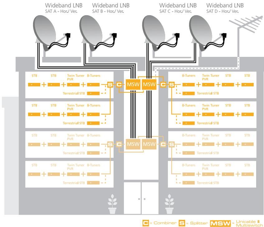
Connect the cables from the Wideband LNBs to the input connectors marked with Sat A/C Vertical and Horizontal and Sat B/D Vertical and Horizontal (pay attention to identification of the Wideband LNB connectors).
