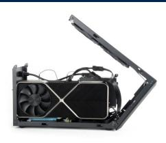
Easy access design with flip-forward top-front panel
