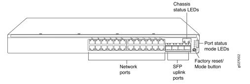
The front panel of an EX2200-C switch consists of the following components:
