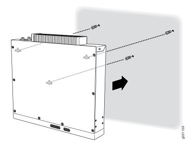
Figure 34: Mounting the EX2200-C Switch on a Wall Using Screws
