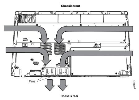
Figure 19: Airflow Through Non-PoE Models of EX2200 Switches Except EX2200-C Switch Models
