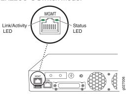
Figure 10: LEDs on the Management Port on an EX2200-C Switch
