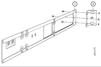
1— Side mounting-rail 2—Front-mounting bracket
