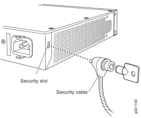
Figure 23: Securing the EX2200-C Switch Using Security Slots
