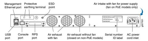
The rear panel of an EX2200-C switch consists of the following components:
