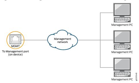
Figure 50: Connecting a Device to a Network for Out-of-Band Management
