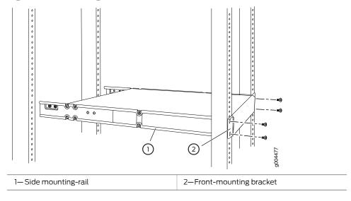
8. Have a second person secure the front of the switch to the rack by using the appropriate screws for your rack.
