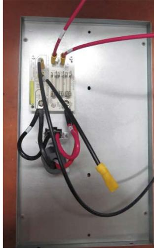
2. Please assemble the 12PCS batteries with black wire into the Battery Case as below.
