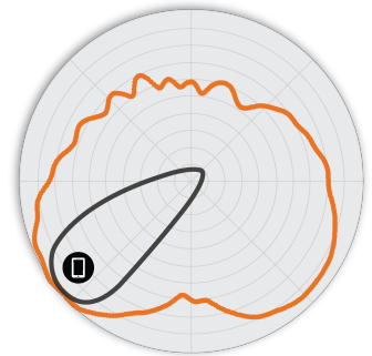
Figure 5. R550 5GHz Elevation Antenna Patterns
