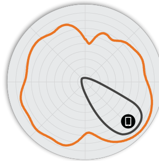
Figure 4. R550 2.4GHz Elevation Antenna Patterns
