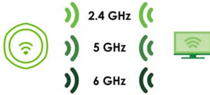
Figure 10 Multi-Link Operation Example
