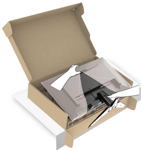
Figure 13. Hold the stand riser and lift the monitor
