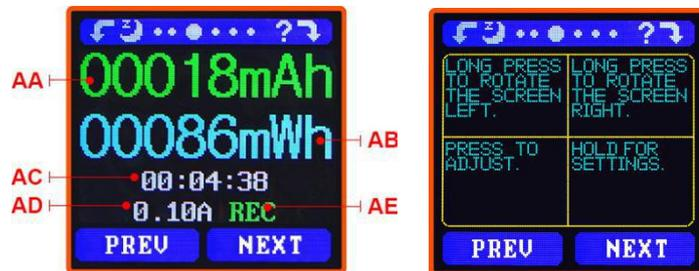
'REC' displayed in red indicates that recording is stopped. 'REC' displayed in green indicates that recording is in progress.
