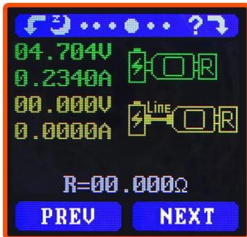
Data Connection Cable Impedance Measurement Interface
