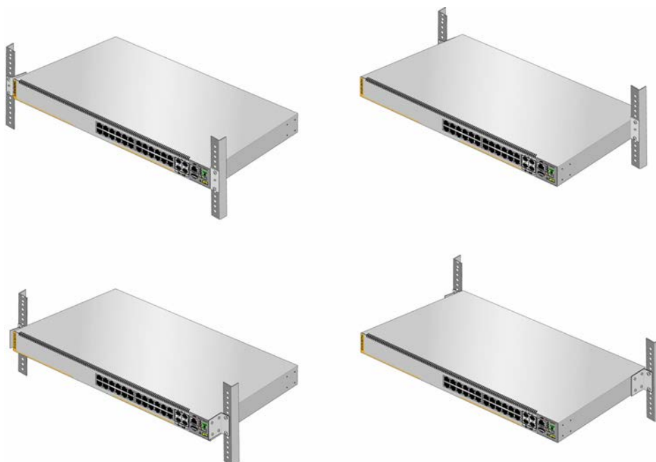
Figure 47. Switch Orientations in an Equipment Rack
