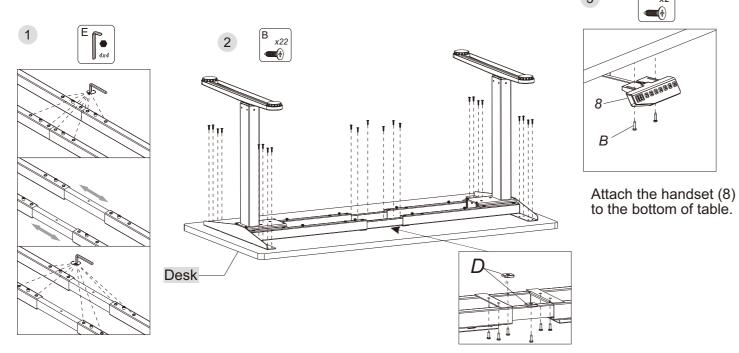
Attach the square washers (D) onto the center of the support beam.
