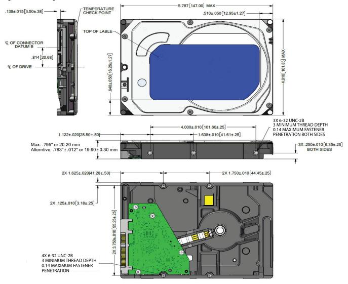
Figure 4 Mounting dimensions (3 and 4-disk models)
