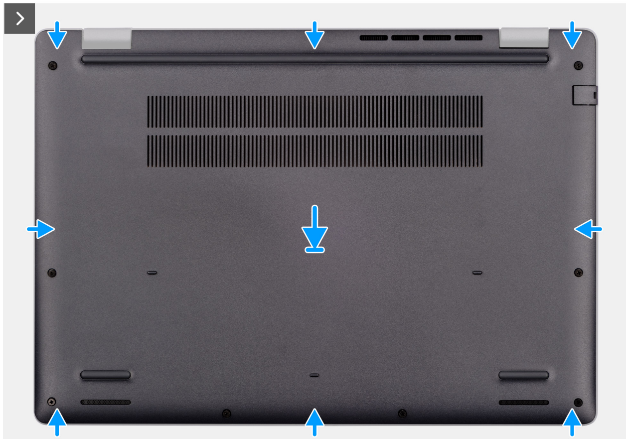
Abbildung 15. Installing the base cover
