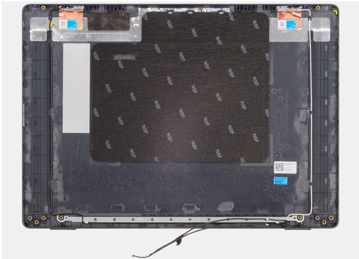
Abbildung 86. Removing the display back-cover assembly
