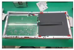
Use a Philips-head screwdriver to remove 9pcs screws for unlocking power board and interface board with the bracket.
