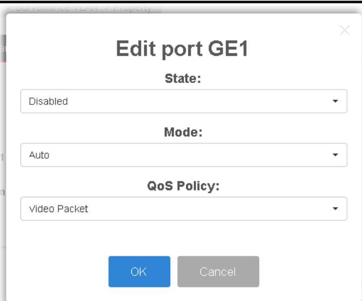
**State** -Set it to enable surveillance VLAN function of interface.
