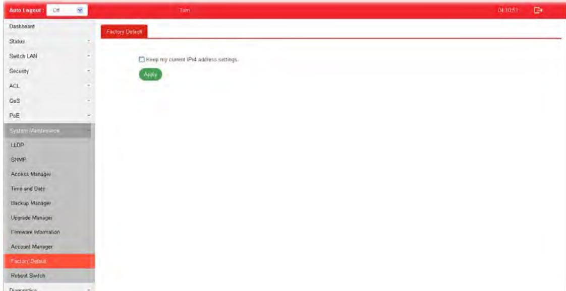
If **Keep my current IPv4 address settings** is checked, after clicking **Apply**, the original configuration for IP address will be kept.
