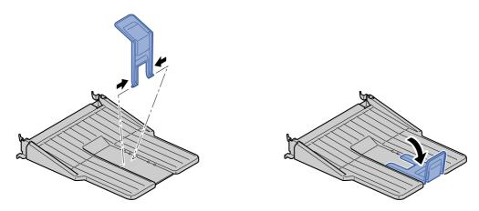
2 Install the Face-up Rear Output Tray on the rear of the machine.
