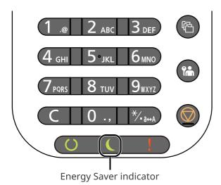
If print data is received during Sleep, the machine automatically wakes up and starts printing.
