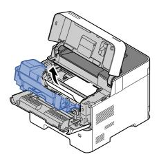
If the jammed paper appears to be pinched by rollers, pull it along the normal running direction of the paper.
