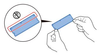
To protect electronic parts, discharge static electricity from your body by touching a water pipe (faucet) or other large metal object before handling the memory modules. Or, wear an antistatic wrist strap, if possible, when you install the memory modules.
