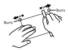
Before loading Hagaki (Cardstock) into the multi purpose tray, fan them and align the edges. If the Hagaki (Cardstock) paper is curled, straighten it before loading. Printing onto curled Hagaki (Cardstock) may cause jams.
