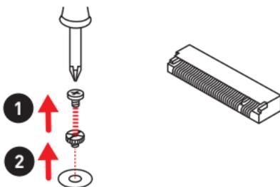
3. Tighten the base screw into the hole of the distance to the M.2 slot as the length your M.2 module.
