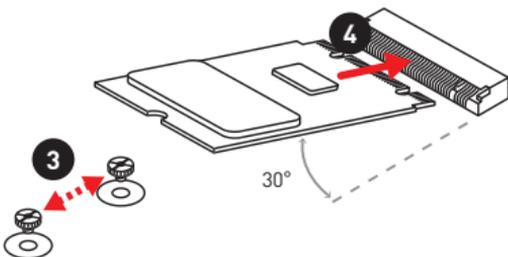
5. Put the screw in the notch on the trailing edge of your M.2 module and tighten it into the base screw.
