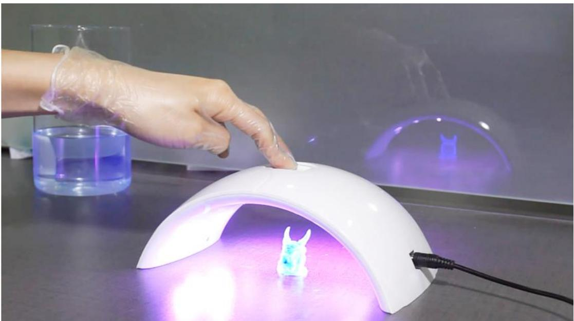
Step14: Irradiate the model with UV-light about 2-3mins.
