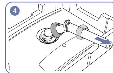
Remove the COVER-REAR TOP after detaching it from the rear cover.
