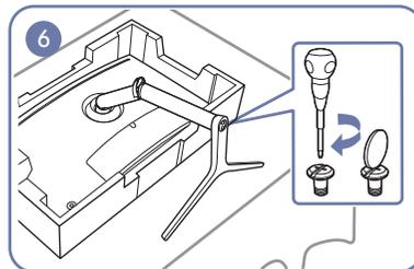
Attach the stand base to the stand neck, and then fasten the two screws on the base to tightly fix it.
