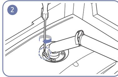
Use the screws on the stand to tightly fasten.
