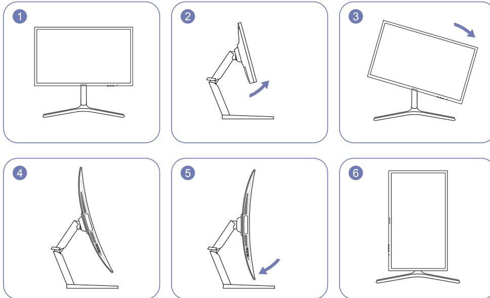
— Adjust the screen following the arrow direction.
