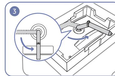
Rotate the stand neck 90° counterclockwise and put the connecting area on the edge of the packaging.
