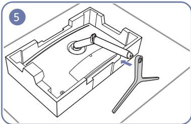
Insert the stand base into the stand neck in the direction shown in the figure.
