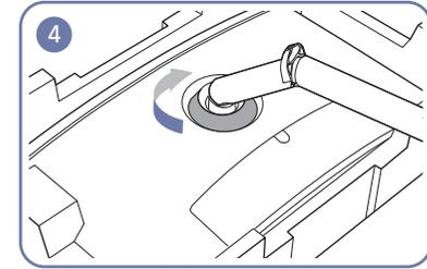
Turn the COVER-REAR TOP clockwise to attach it to the rear cover.
