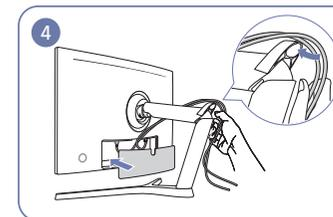
Run the cables through the holder in the direction of the arrow from the lower part of the holder, as shown in the image.
