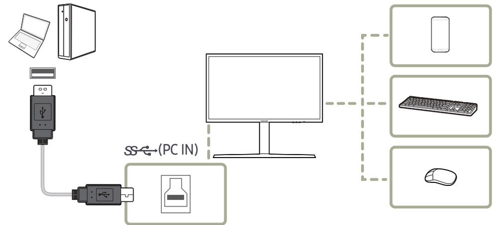
If multiple source devices are connected to the PC, the many cables around the PC may look messy. Connecting the devices directly to the product will resolve such inconvenience.
