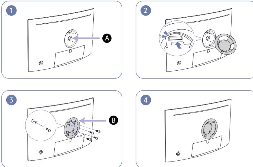
**A** Attach the BRACKET WALL here
