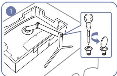
Place the screen on the Styrofoam or soft cushion included in the package, hold the stand base with one hand and remove the screws of the stand base with another hand.
