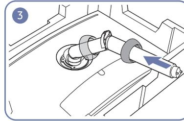
Attaching the COVER-REAR TOP to the stand neck, as shown in the figure.
