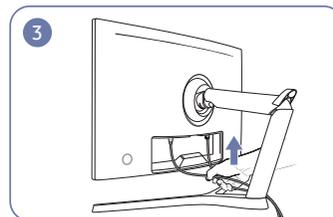
Connect cables to the appropriate connectors.
