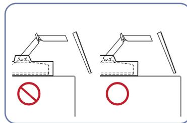
Keep the stand base within the platform to prevent it falling off and causing injury.
