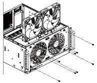
2. Secure the radiator assembly on to the front panel
