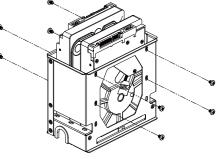
2. Install Nvidia 30 series graphics card bracket (slightly tighten the screws, and reserve space for the bracket to slide left and right
