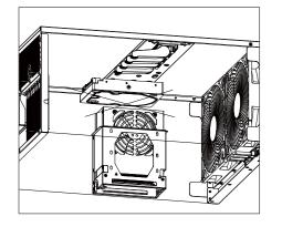
2. Install 120mm, 240mm or 360mm radiator on the bracket
