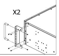
2. Install handle bar onto the flat handle bar bracket
