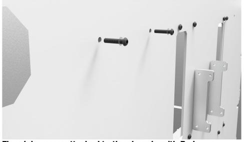
The pinions are attached to the chassis with 2 pieces of M4x30mm screws along with silicon pads from the backside.
