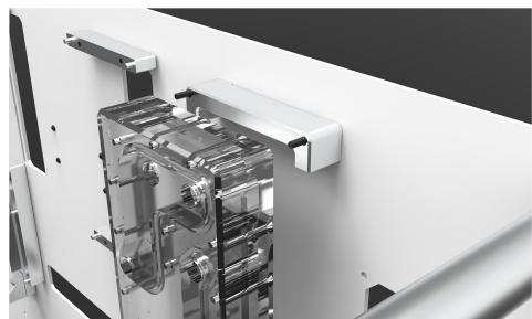
Gently press the acrylic Pinion towards the screws while simultaneously tightening the screws from the backside. Take care no to tighten too hard as the acrylic might crack.
