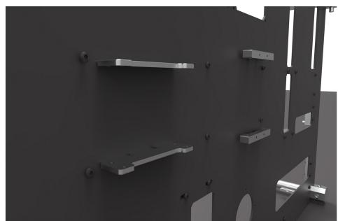
Later on, tighten rest of screws, carefully check if all of them are settled correctly.
