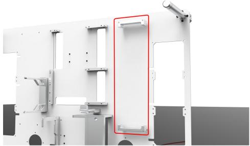
The picture above shows how the brackets should be placed.
