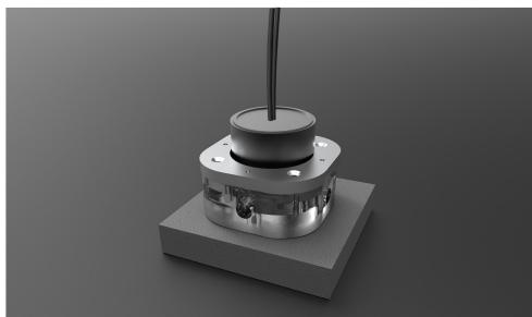
Carefully lie down our aluminium base. There will be wires going from 05 pump - they have to be inside of hole in aluminium base.
