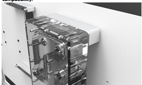
The screws are only to be tightened so that there are no gap between the acrylic and aluminum and the aluminum and the chassis.
