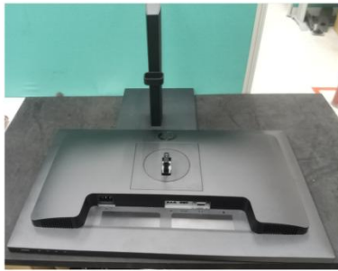
2.2 Remove stand base assembly
