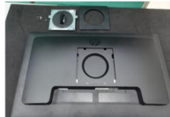
3.2 Release the hinge screw and remove the hinge
