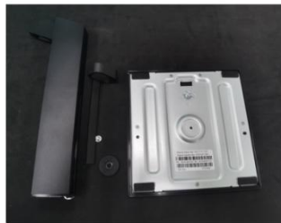
7.2 Remove the base, rubber and cable holder
