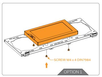
There are many ways to install your EK-Quantum Lumen 7"LCD screen as it utilizes a standard mounting hole pattern (105 mm), the same as all EK Fans.
