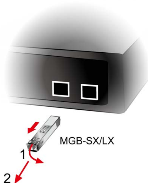
Figure 2-10: How to Pull Out the SFP/SFP+ Transceiver
