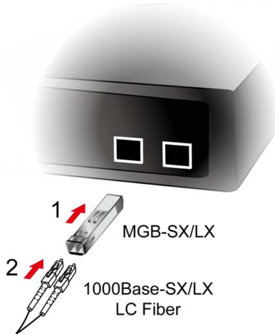
Figure 2-9 Plug in the SFP transceiver
