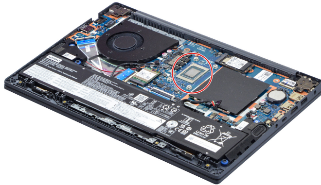
Figure 4. Areas on the system board where thermal interface materials are applied
