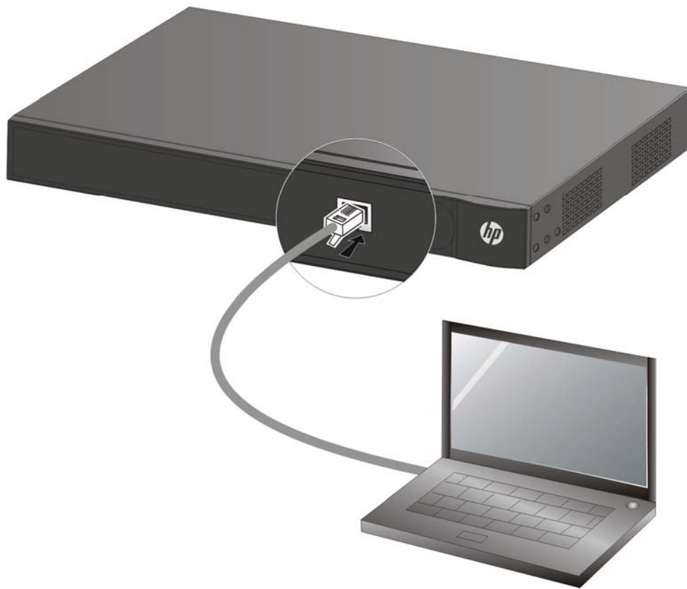
Figure 152 Connecting a Workstation to the switch using the Console Port
