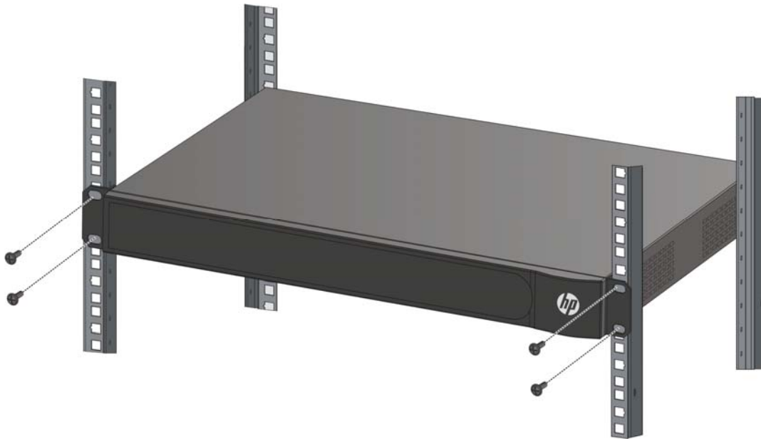
Figure 50 Mount the HP V1905 Switch to a rack
