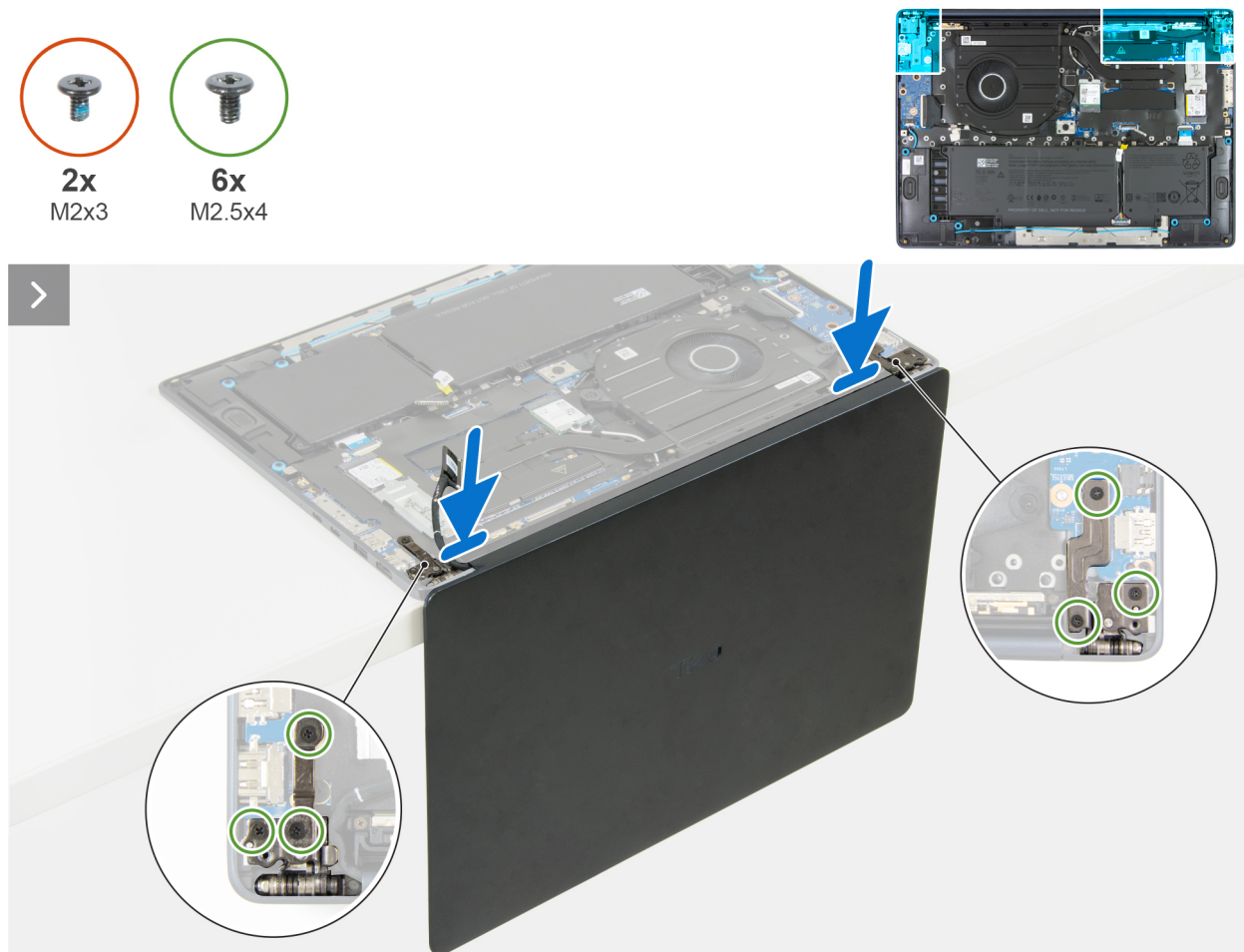
Figure 24. Installing the display assembly
