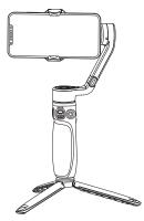
G Before the calibration, please make sure the gimbal is straightly put on a flat surface. Please don't touch the gimbal when in calibration.
