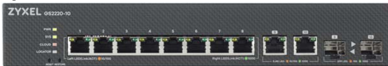
Figure 12 Front Panel: GS2220-10HP
