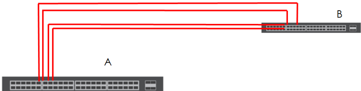
Figure 150 Trunking Example – Physical Connections
