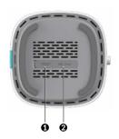
1. Reset button 2. Nano Sim card slot 3. USB 3.0 4. 2.5 Gigabit Ethernet Port (WAN/LAN) 5. Gigabit LAN Ethernet Port 6. Phone Port (RJ11) 7. On/Off button 8. Power Supply connector
