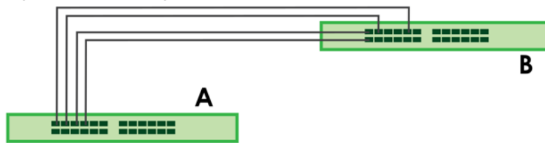
Figure 146 Trunking Example – Physical Connections
