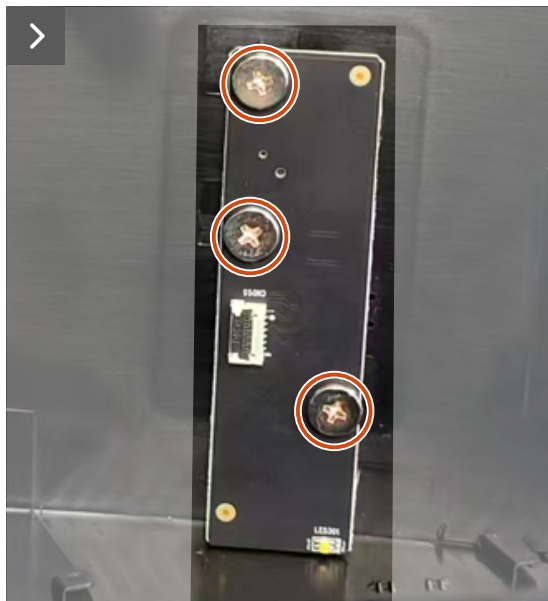
Figure 20. Installing the keypad board
