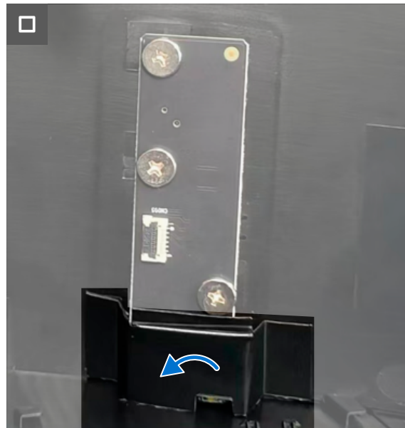
Figure 20. Installing the keypad board
