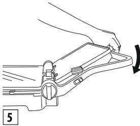
Lifting the handgrip slightly before pulling the release lever lightens pressure on the hinge and facilitates the operation. The appliance can be used as a grill/barbecue to prepare hamburgers, steak, chicken and fish. The grill/barbecue mode is the most versatile. The grill plates are in the open position, doubling the cooking surface (see figure 6).
