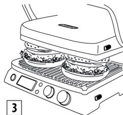
The grease from the food is drained and collected by the grooves on the plate and the hole at the back and is collected in the grease tray.
