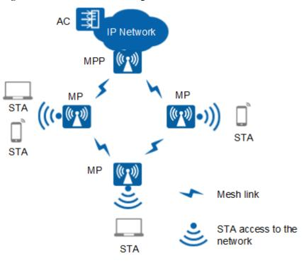
Figure 1-4 Fit AP mesh networking
