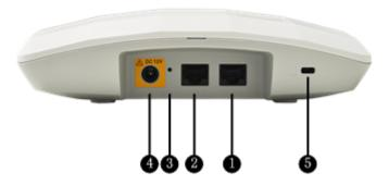
As shown in Figure 2-4, the AP has the following interfaces.
