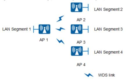
In this networking, the AP connects two or more independently wired or wireless LANs through wireless links to construct a network on which users can exchange data. In Wireless Distribution System (WDS) mode, the AP supports point-to-point (P2P) and point-to-multipoint (P2MP) networking modes. Supporting 5 GHz and 2.4 GHz frequency bands, the AP can implement wireless bridging and access functions.
