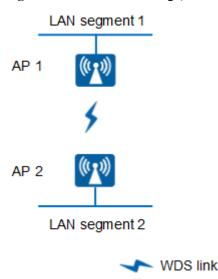
Figure 1-2 Fit AP networking (WDS mode: point-to-point)
