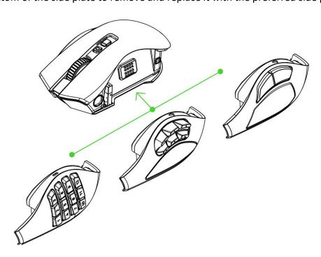
Unplug the mouse before changing a side plate. These side plates are exclusively designed for the Razer Naga V2 Pro. Don't use side plates designed for other Razer products and vice versa.
