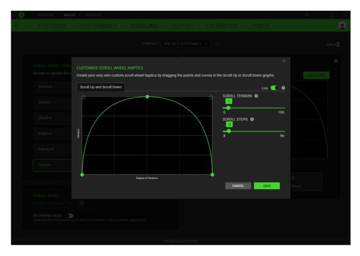
You can modify the scroll up and down haptics by directly tweaking any of the points in the curve or by adjusting the scroll tension and steps slider.
