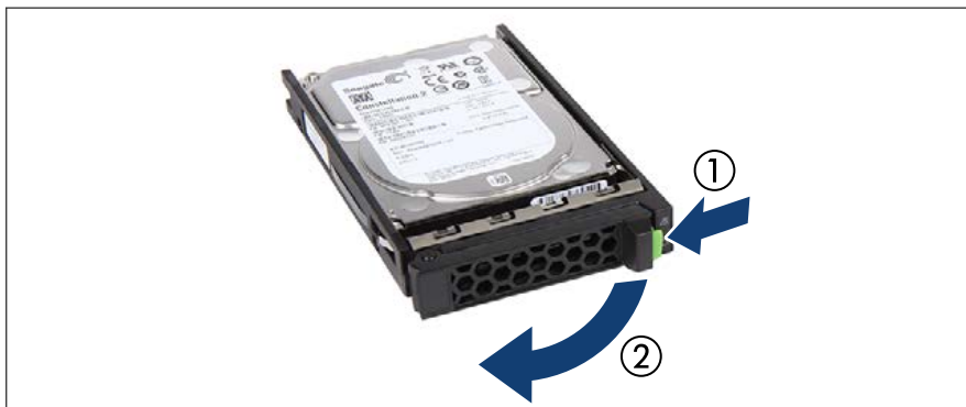
Figure 85: Opening the locking lever
