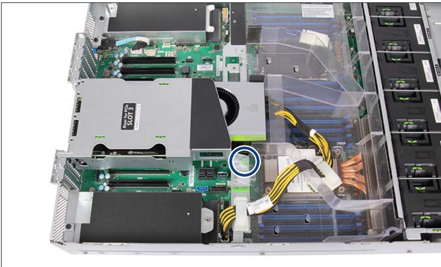
Figure 24: Removing the riser module 1
