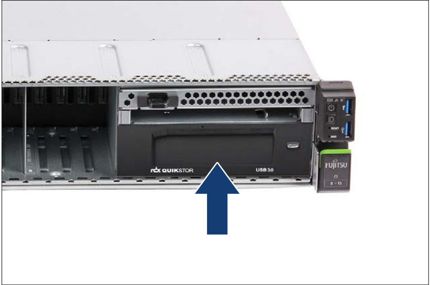
Figure 293: Installing the RDX drive (B)
