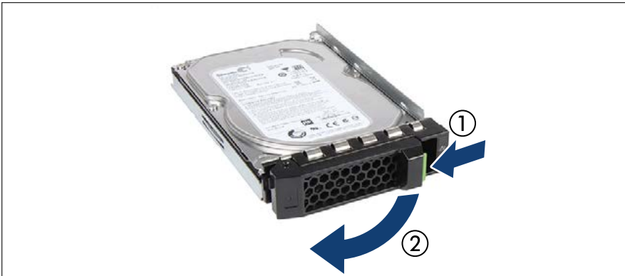
Figure 64: Opening the locking lever
