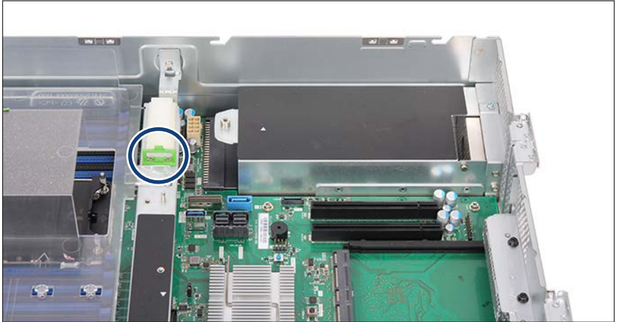
Figure 246: Storing the ODD latch
