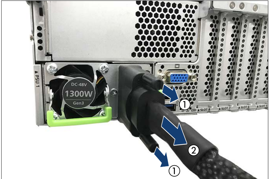
Figure 6: Disconnecting the server from the dc voltage - example DC PSU -48 V
