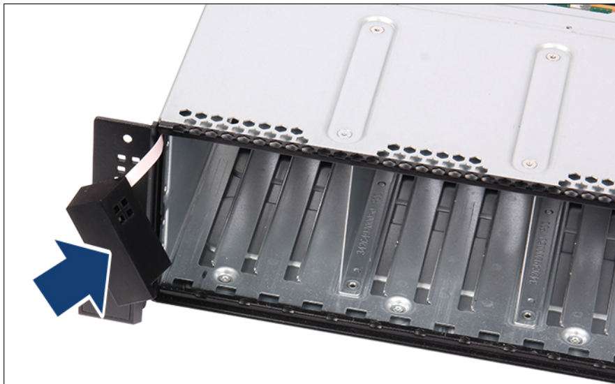
Figure 308: Installing the thermal sensor
