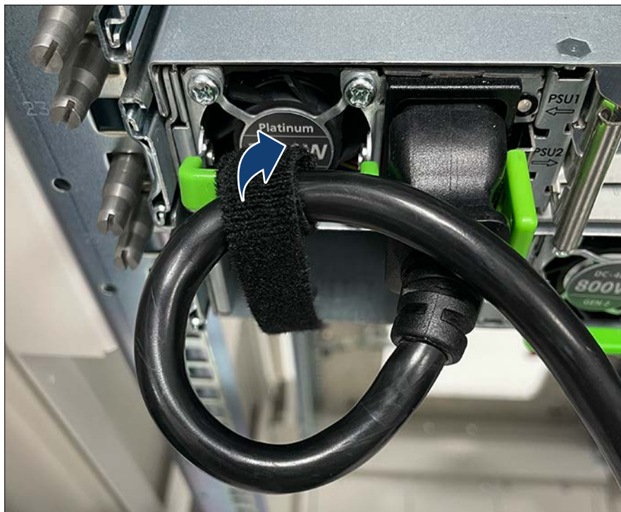
Figure 5: Loosening the hook-and-loop tape
