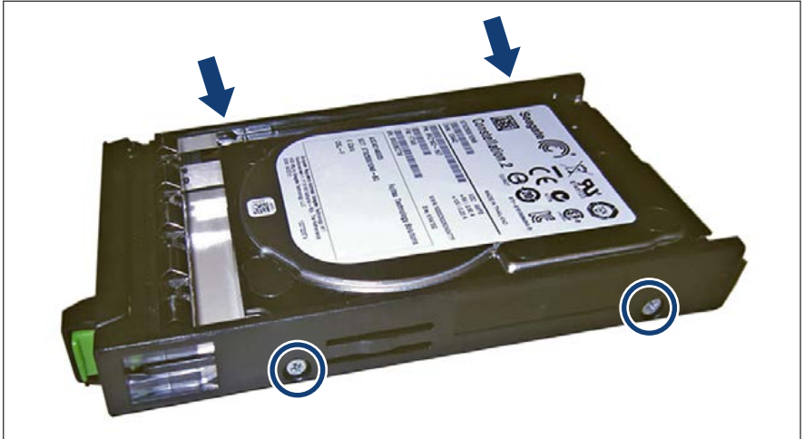
Figure 55: Installing the 2.5-inch HDD/SSD in the 2.5-inch installation frame (B)
