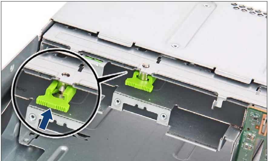
Figure 294: Installing the RDX drive (C)
