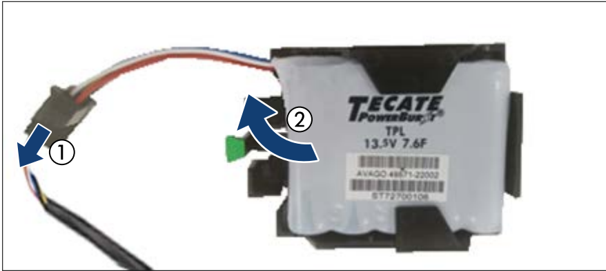
Figure 192: Removing the FBU from the holder
