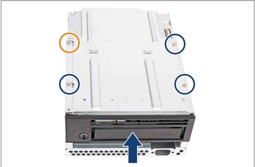
Figure 276: Installing the LTO drive (A)
