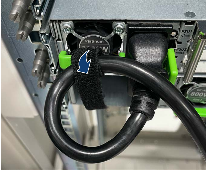
Figure 19: Securing the power cord with the hook-and-loop tape (B)
