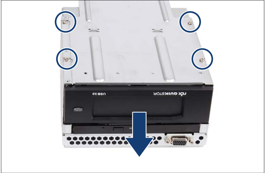
Figure 299: Removing the RDX drive (C)
