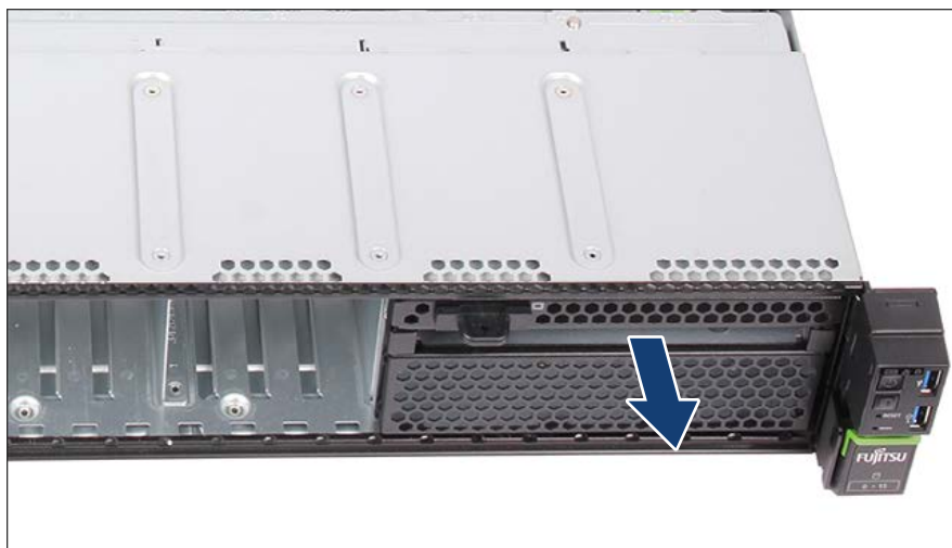
Figure 247: Removing the dummy cover
