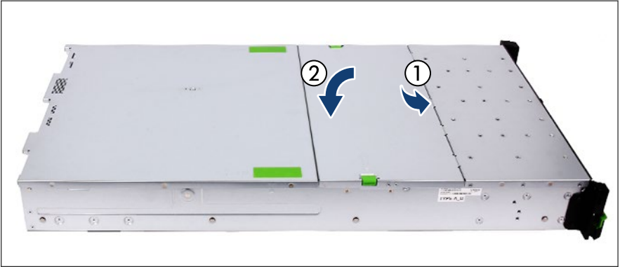
Figure 13: Installing the top cover 1
