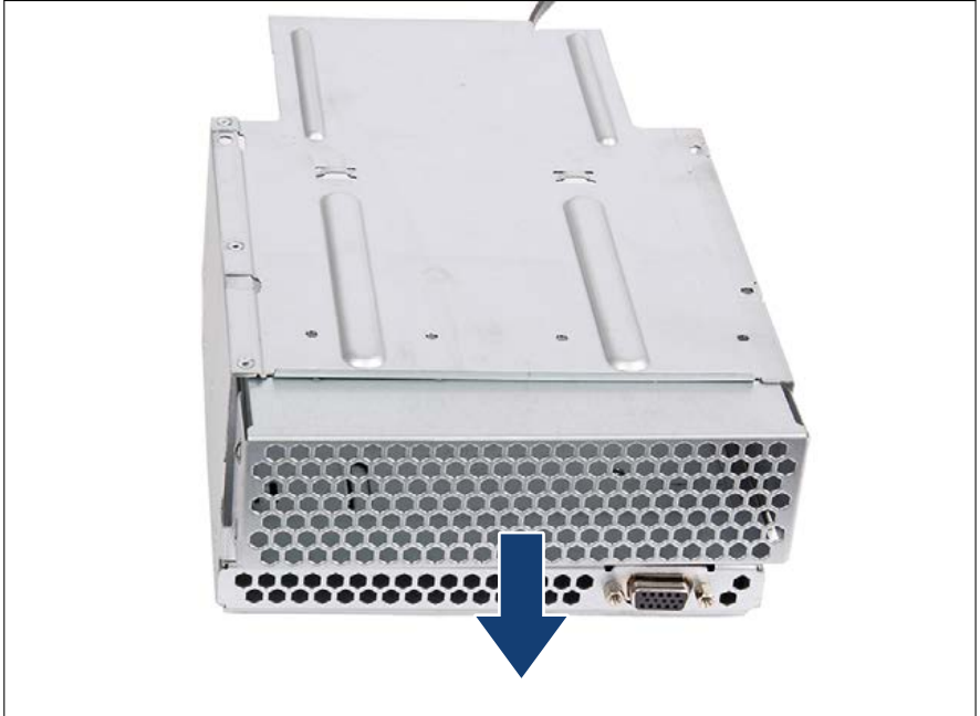
Figure 291: Removing the air grid (B)
