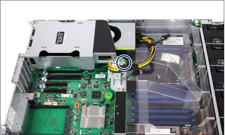
Figure 27: Installing the riser module 2
