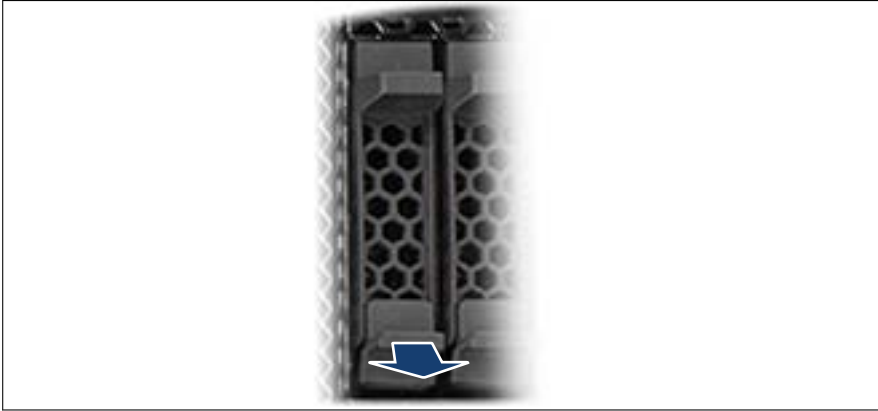
Figure 78: Removing the dummy lock
