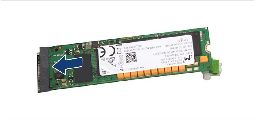
Figure 107: Installing the M.2 SSD (A)
