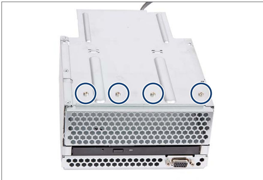
Figure 290: Removing the air grid (A)
