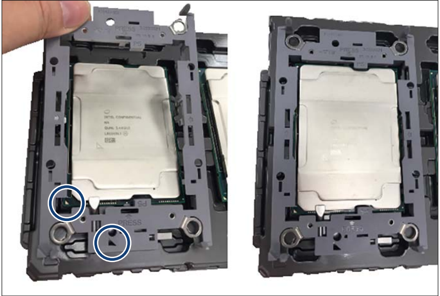
Figure 215: Installing the CPU frame on the CPU
