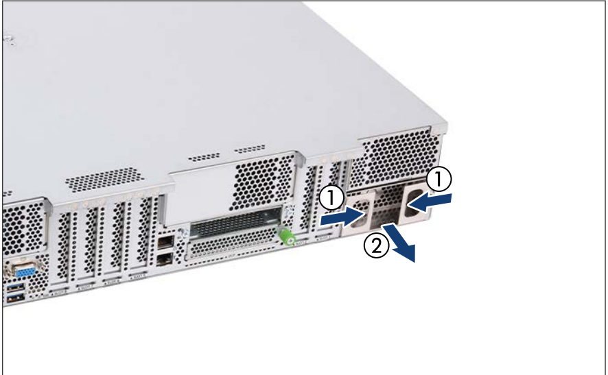
Figure 46: Removing the dummy cover
