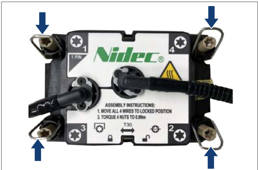
Figure 233: Removing the LC heat sink (B)
