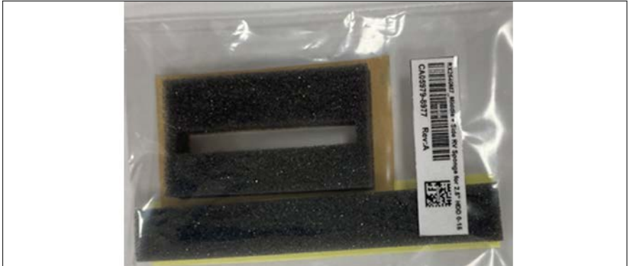
Figure 90: Foams for the 8x 2.5-inch HDD backplane
