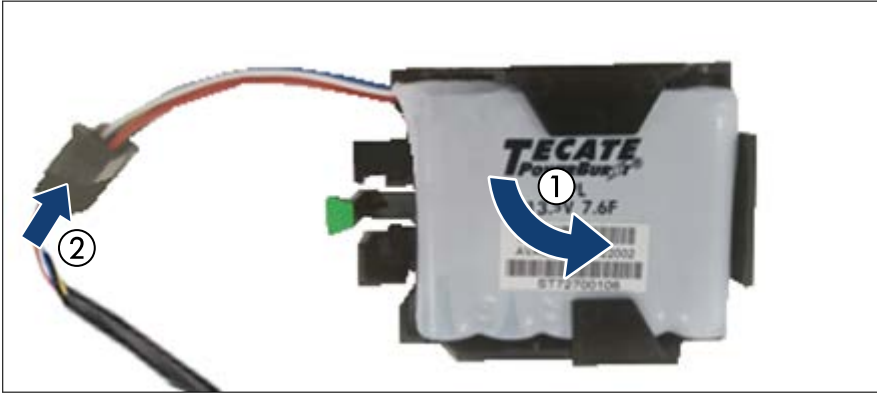
Figure 188: Installing the FBU in the holder
