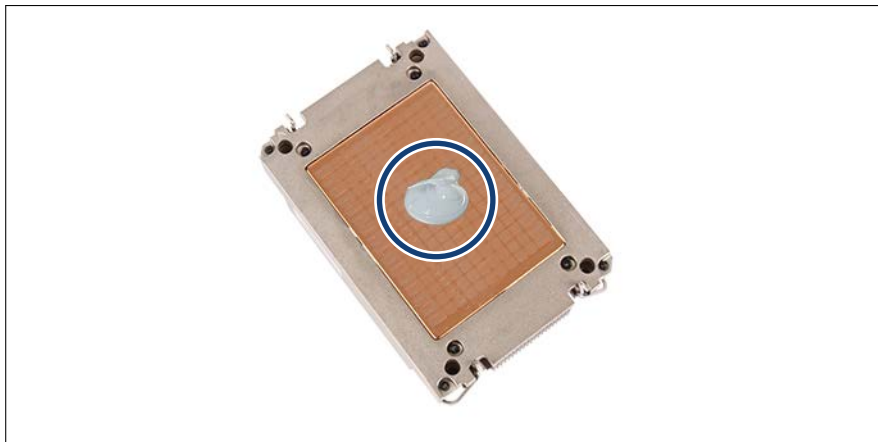
Figure 229: Applying the thermal paste
