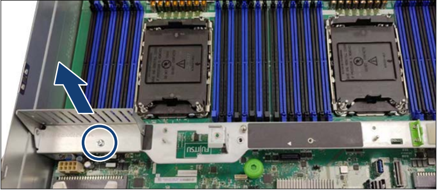
Figure 161: Removing the GPU dummy bracket
