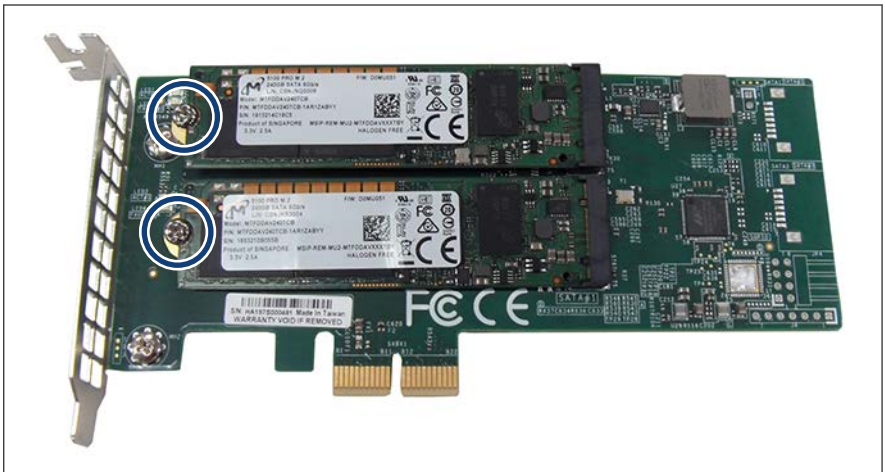
Figure 155: Installing M.2 SSDs (B)
