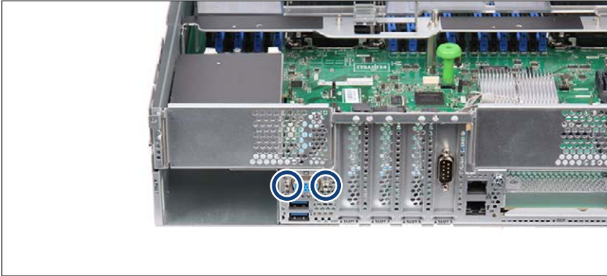
Figure 328: Removing the rear VGA connector (A)
