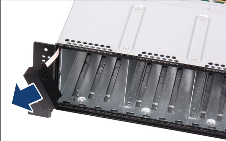
Figure 306: Removing the thermal sensor
