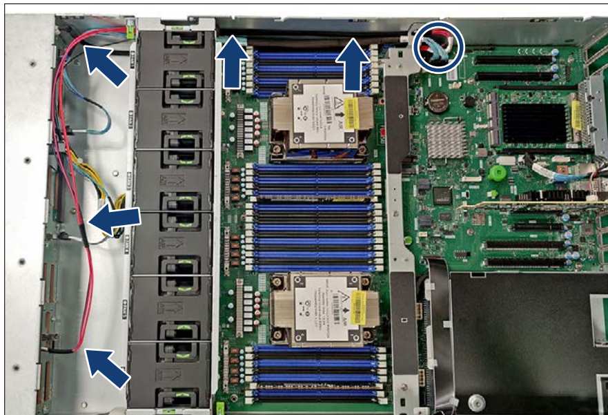
Figure 263: Routing of the ODD cable to the system board
