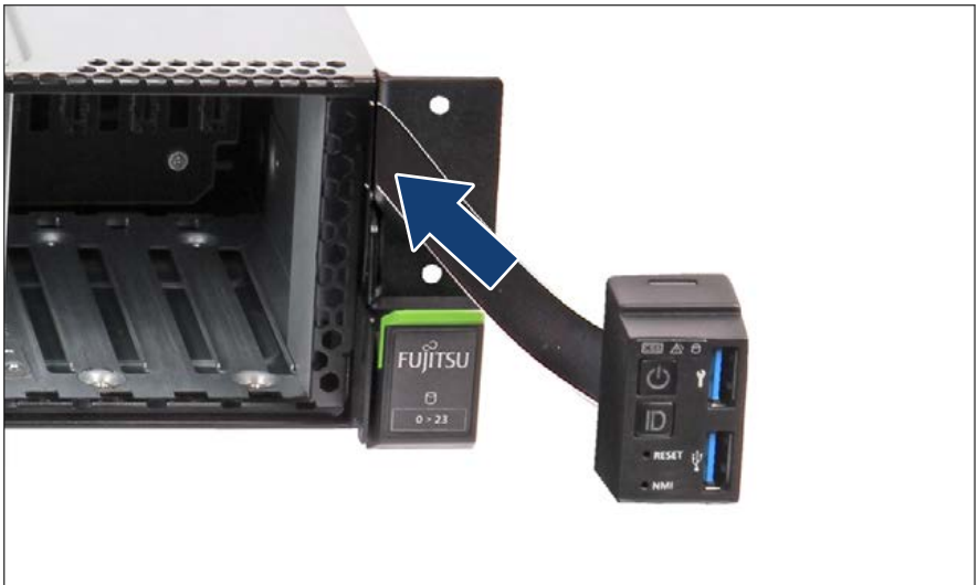
Figure 314: Installing the COP (B)
