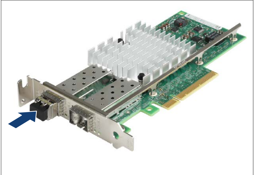
Figure 137: Installing the protective cap
