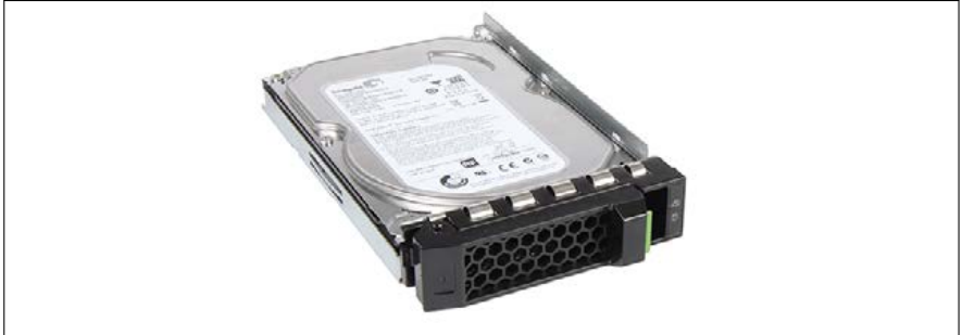
Figure 52: Installing the 3.5-inch HDD in the 3.5-inch installation frame (A)
