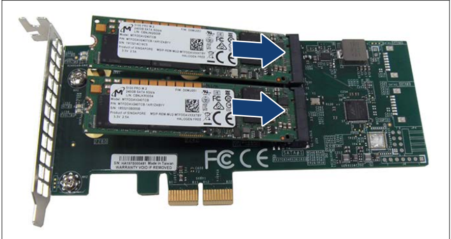
Figure 154: Installing M.2 SSDs (A)
