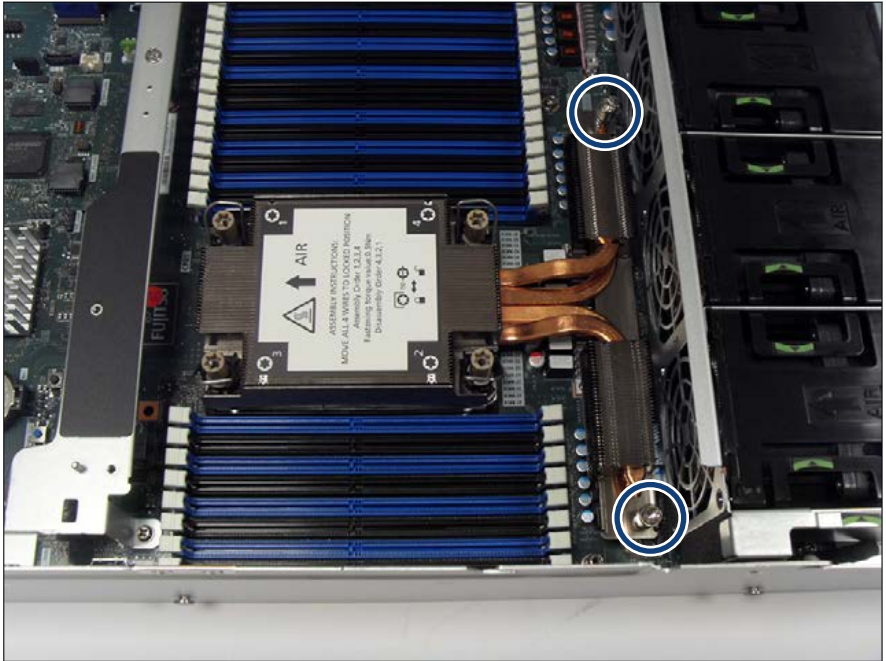
Figure 224: Removing an EVAC CPU heat sink
