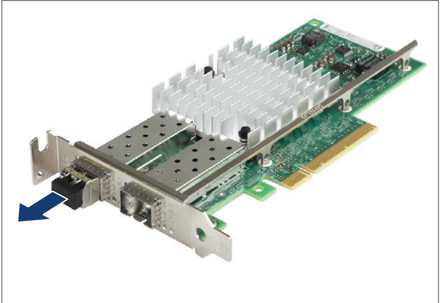
Figure 139: Removing the protective cap
