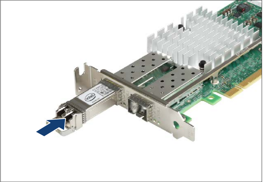
Figure 135: Inserting the SFP+ transceiver module
