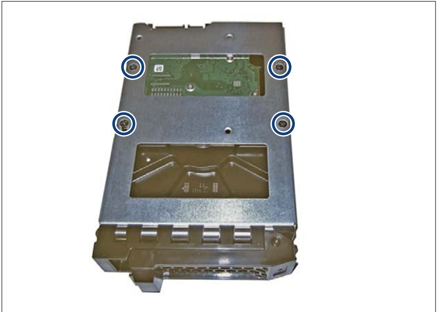
Figure 53: Installing the 3.5-inch HDD in the 3.5-inch installation frame (B)
