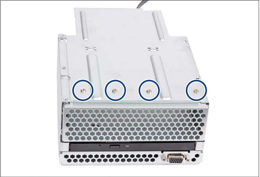
Figure 274: Removing the air grid (A)
