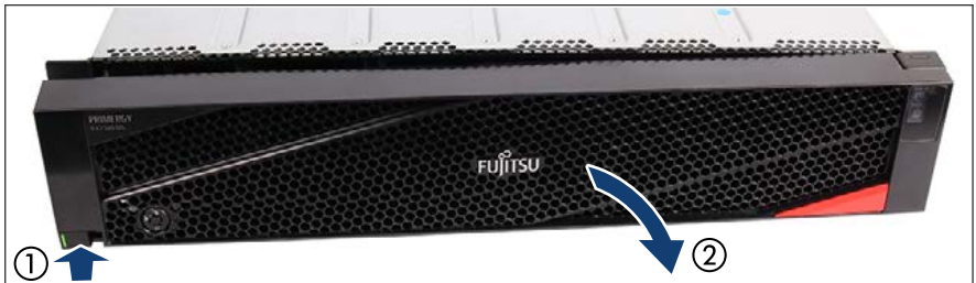
Figure 3: Removing the front cover
