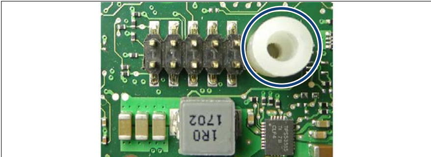
Figure 336: Inserting the TPM spacer on the system board
