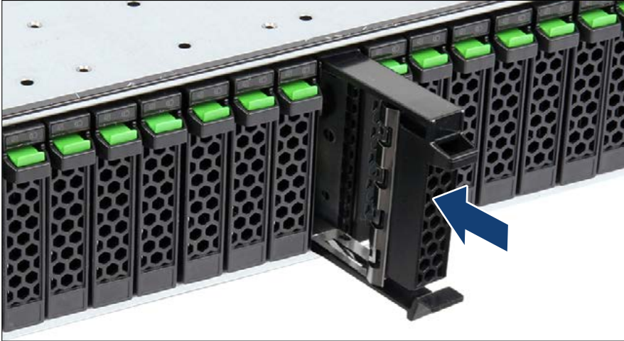
Figure 88: Installing the 2.5-inch HDD/SSD dummy module
