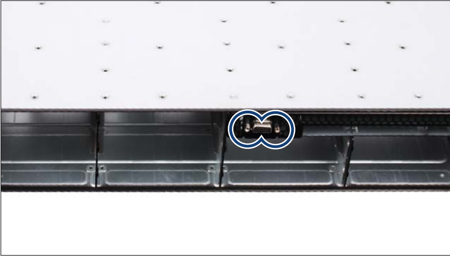
Figure 320: Removing the front VGA
