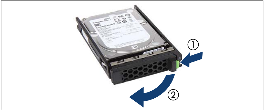
Figure 87: Opening the locking lever
