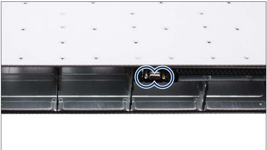
Figure 318: Installing the front VGA
