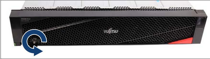
Figure 23: Turning the key
