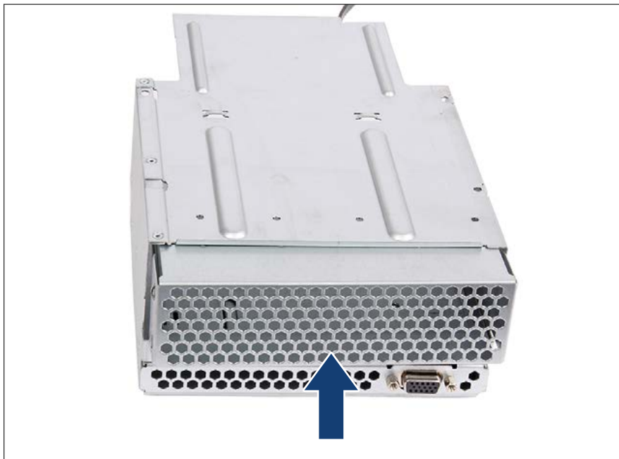
Figure 300: Installing the air grid (A)
