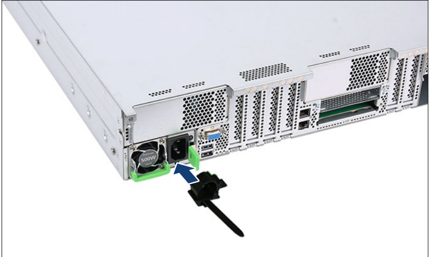
Figure 48: Installing the cable clamp
