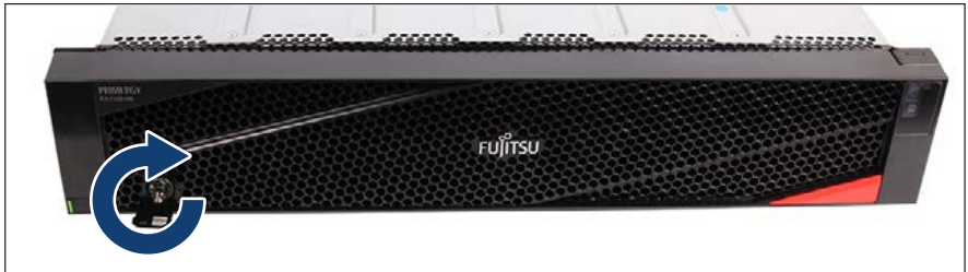
Figure 2: Turning the key
