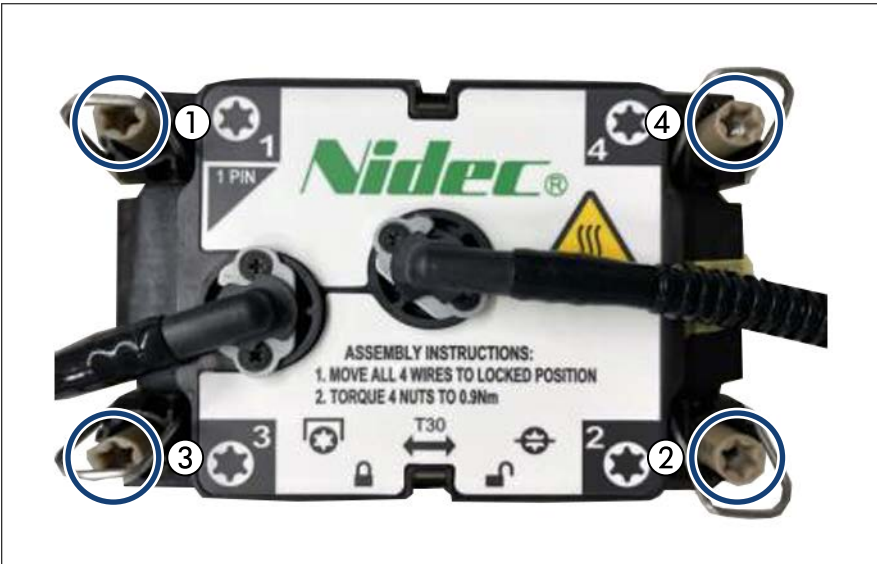
Figure 232: Removing the LC heat sink (A)
