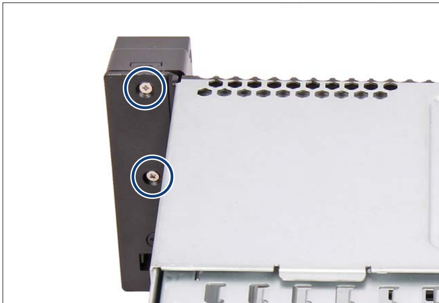
Figure 312: Removing the COP (A)
