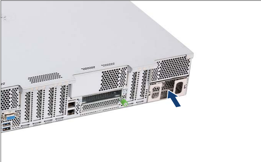
Figure 51: Installing the dummy cover
