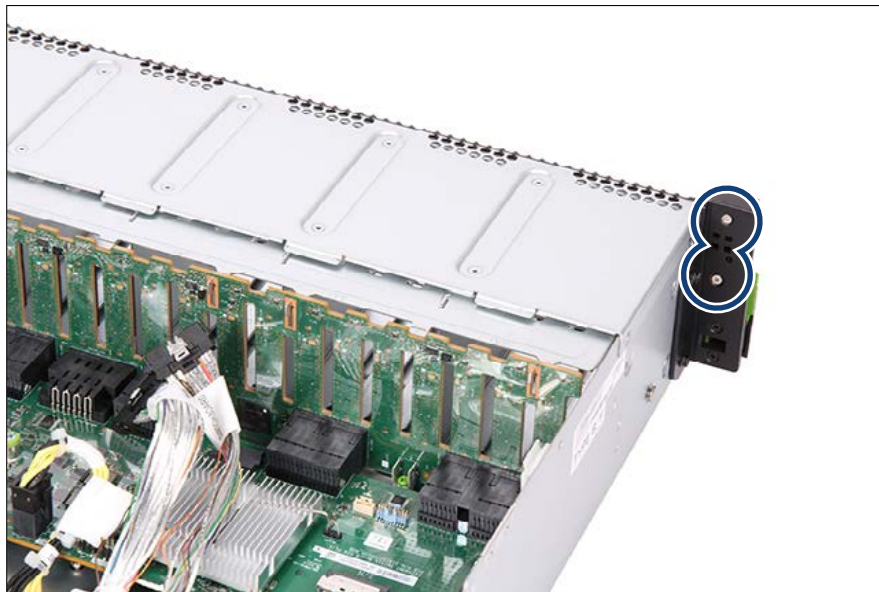
Figure 310: Fasten the thermal sensor
