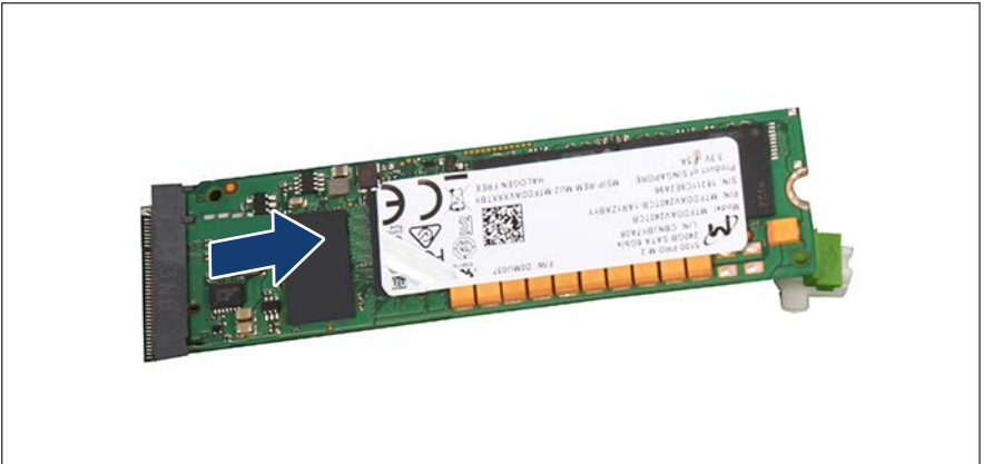
Figure 110: Removing the M.2 SSD (B)
