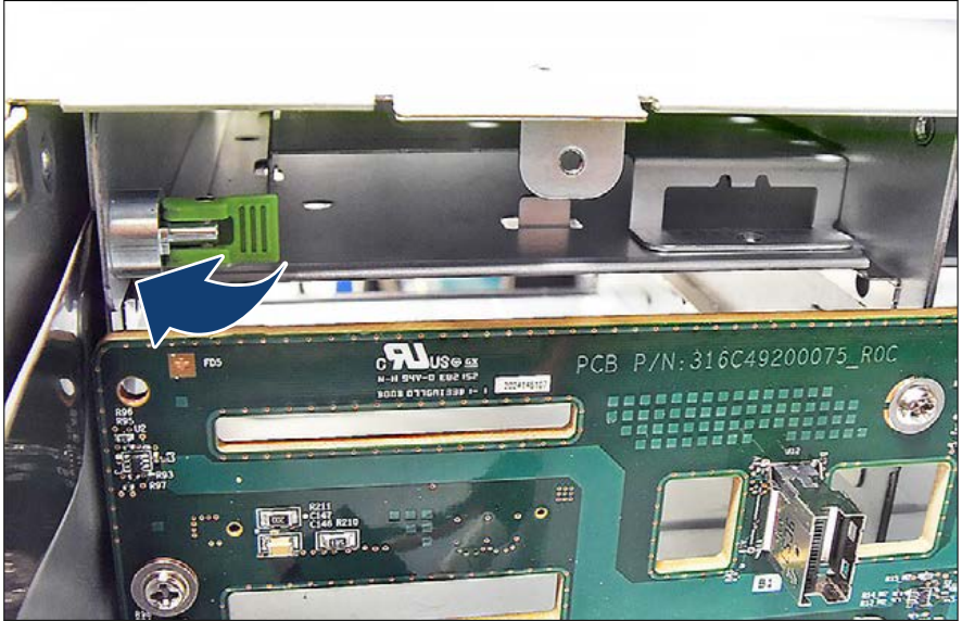
Figure 269: Locking the ODD cage
