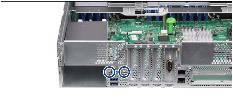
Figure 331: Installing the rear VGA connector (B)
