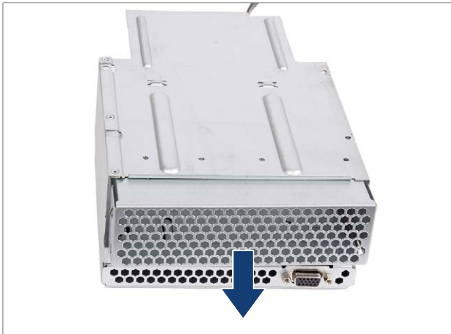
Figure 275: Removing the air grid (B)
