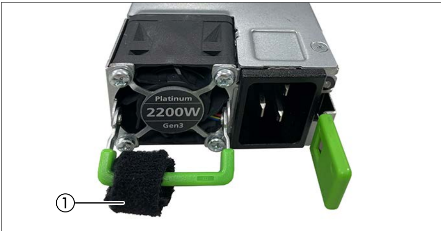
Figure 17: Example PSU with hook-and-loop tape
