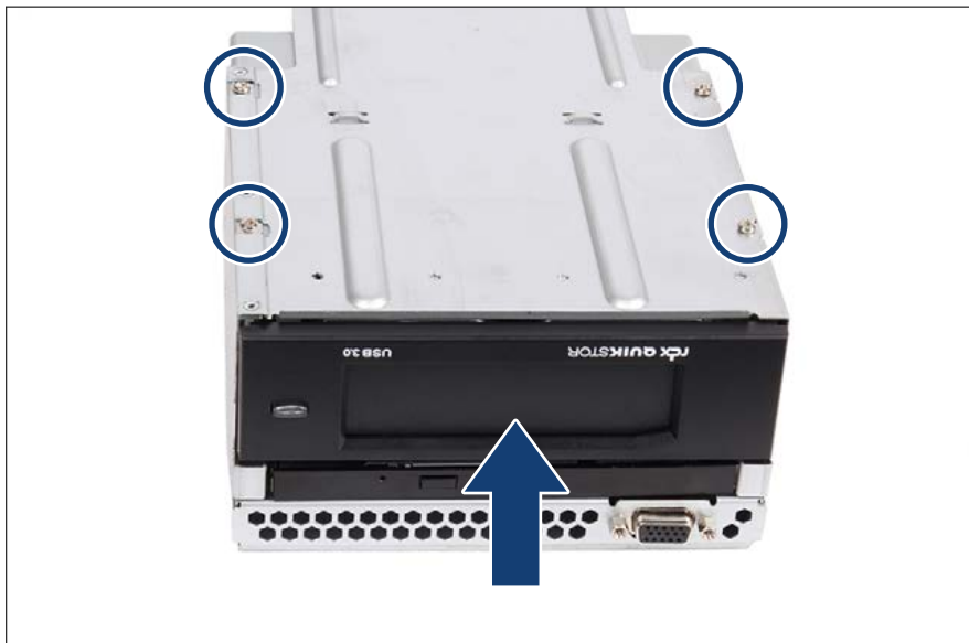
Figure 292: Installing the RDX drive (A)
