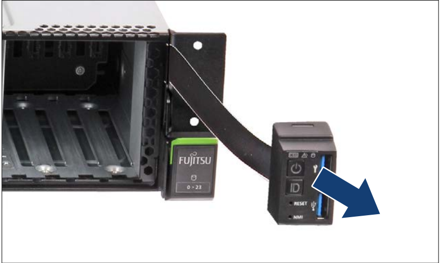
Figure 313: Removing the COP (B)
