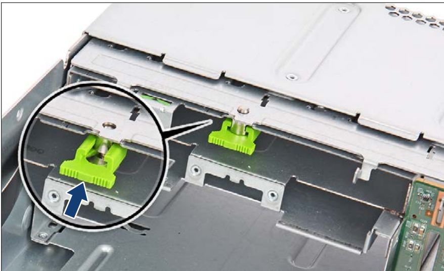
Figure 278: Installing the LTO drive (C)
