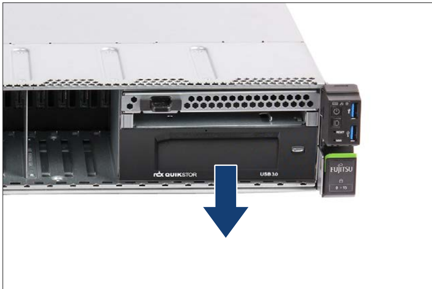
Figure 298: Removing the RDX drive (B)
