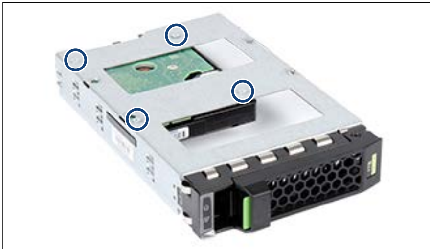
Figure 57: Installing the 2.5-inch HDD/SSD in the 3.5-inch installation frame (B)
