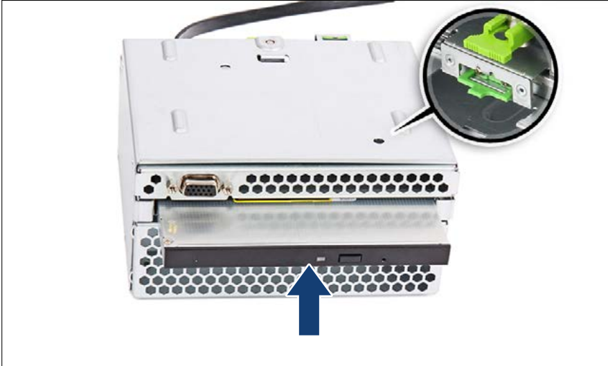
Figure 249: Installing the ODD
