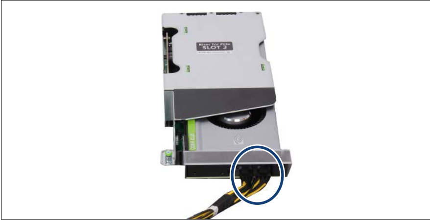
Figure 159: Connecting the GPU power cable
