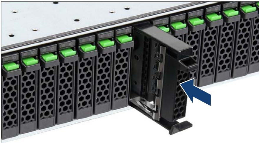
Figure 82: Installing the 2.5-inch HDD/SSD dummy module
