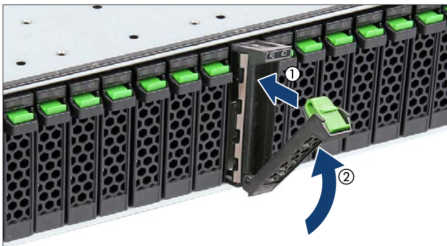
Figure 86: Installing the 2.5-inch PCIe SSD module
