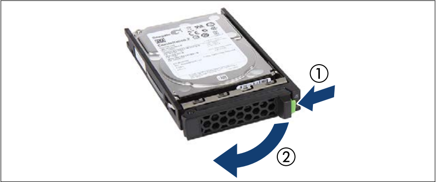
Figure 80: Opening the locking lever
