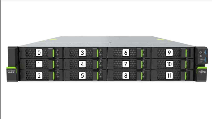
Figure 61: Configuration with up to 12 3.5-inch HDD modules
