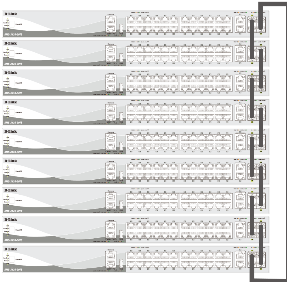
Figure 4-69 Duplex Ring stacking topology (SFP28 ports)
