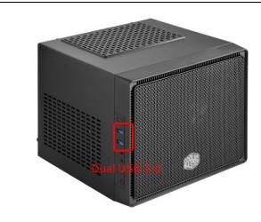
Full mesh front panel and perforated side/top panels for optimized cooling
