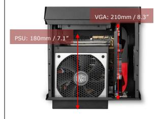
Supports **PSU** up to 180mm & **VGA** up to 210mm
