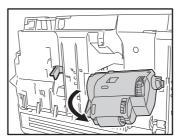
5 Attach the right joint of the new feed roller.
