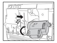
Raise the feed roller toward the back until the securing lever clicks into place.
