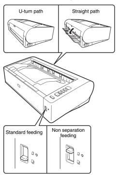
Standard feeding is used when the feed selection lever at the front of the scanner is lowered, and non separation feeding is used when it is raised. Standard feeding is used to feed documents one page at a time. Non separation feeding is used to feed bound or fastened multi-page documents or folded documents without separating them.
