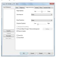
Set the processing method for scanned images.
