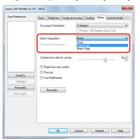
When [Batch Separation] is set to [Auto], the batch is separated after the next document is placed and scanning is continued. When [Patchcode] is set, batch separation can be performed by using a patchcode. (See p. 43)
