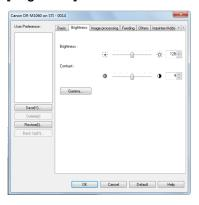
Adjust the brightness and contrast of scanned images. In addition, you can also click [Gamma] and set the gamma correction value for scanned images.
