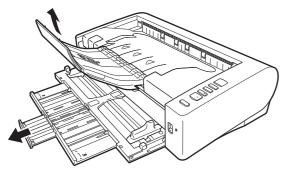
5 Adjust the document guides to fit the width of the document to be scanned.
