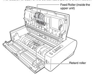
Close the upper unit by gently pushing down on the left and right sides. Push until it clicks into place to make sure that it is completely closed.
