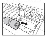
Slide the securing lever for the retard roller to the right, and lower it backward.
