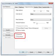
Select the [Erase Dot] check box to automatically remove isolated black dots (3 x 3 dot size) from white backgrounds (or white dots from black backgrounds).  Select the [Erase Notch] check box to remove notches that protrude from object outlines in scanned images.
