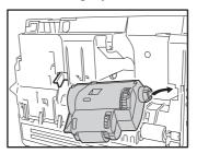
Attach the left side of the feed roller, and slide the securing lever for the feed roller to the right.
