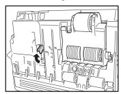
Slide the securing lever for the feed roller to the left.
