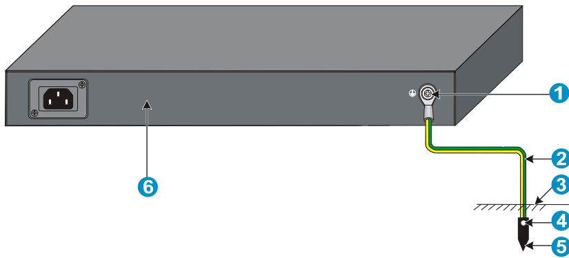
Figure 26 Ground the switch by burying the grounding conductor into the earth ground
