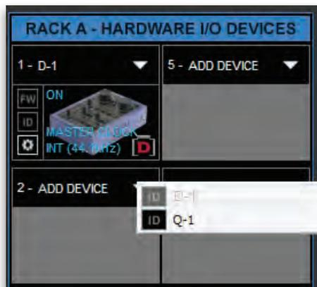
In this example the DiGiGrid **D** is the SoundGrid network's clock master device, indicated by its blue color and the icon text: On, Master Clock, INT (48 kHz).
