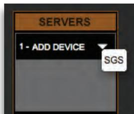
A server cannot be shared by multiple SoundGrid host applications such as SoundGrid Studio or MultiRack. Within a SoundGrid network, only one computer can utilize a server's processing power for StudioRack and the eMotion ST mixer. Once assigned to a computer, a server remains unavailable to all other computers until released by the user.
