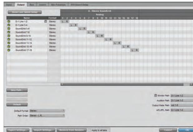
In the Patch page (left), DiGiGrid **D** analog channels 1–4 are patched to driver channels 1–4. The arrow on the upper left of the Patch indicates that signal flows from the DiGiGrid **D** to the driver. Now look at the DAW I/O. The 4 driver channels appear at the top, and are patched to DAW input channels 1-4.
