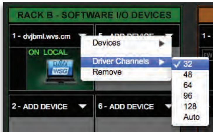
When you configure your host application, you can allocate between Auto, 32, and 128 driver channels. This is done in Rack B of the Setup page. The number of channels you select here is reflected in the Patch page: fewer allocated channels means fewer channels visible.
