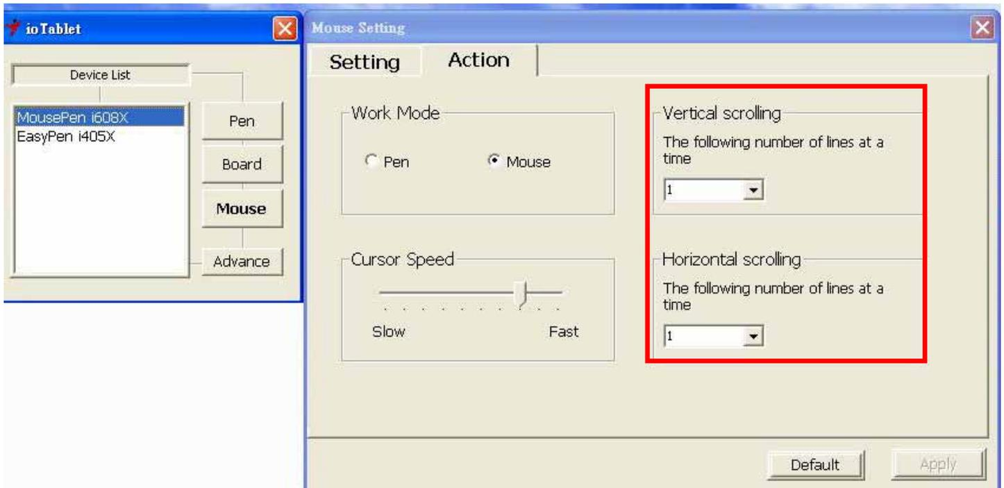
The mouse wheel support vertical and horizontal scrolling, you may set up the number of line at a time while scrolling from 1 to 3 lines.
