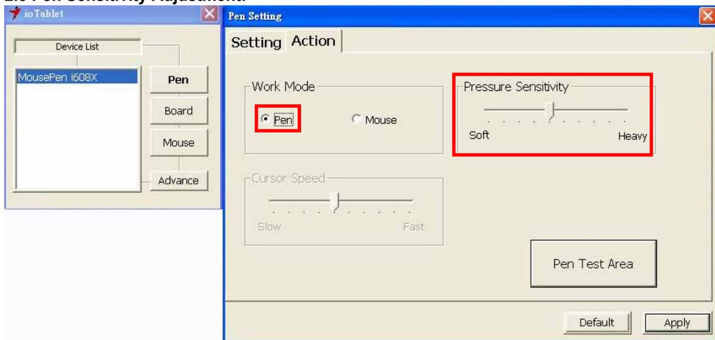
This tablet pen offers 1024 pressure levels sensitivity for all kinds of shapes and thickness. Move the slider in the sensitivity bar to adjust the levels. There is a test area to draw a line by pressing the pen tip on the tablet pad.
