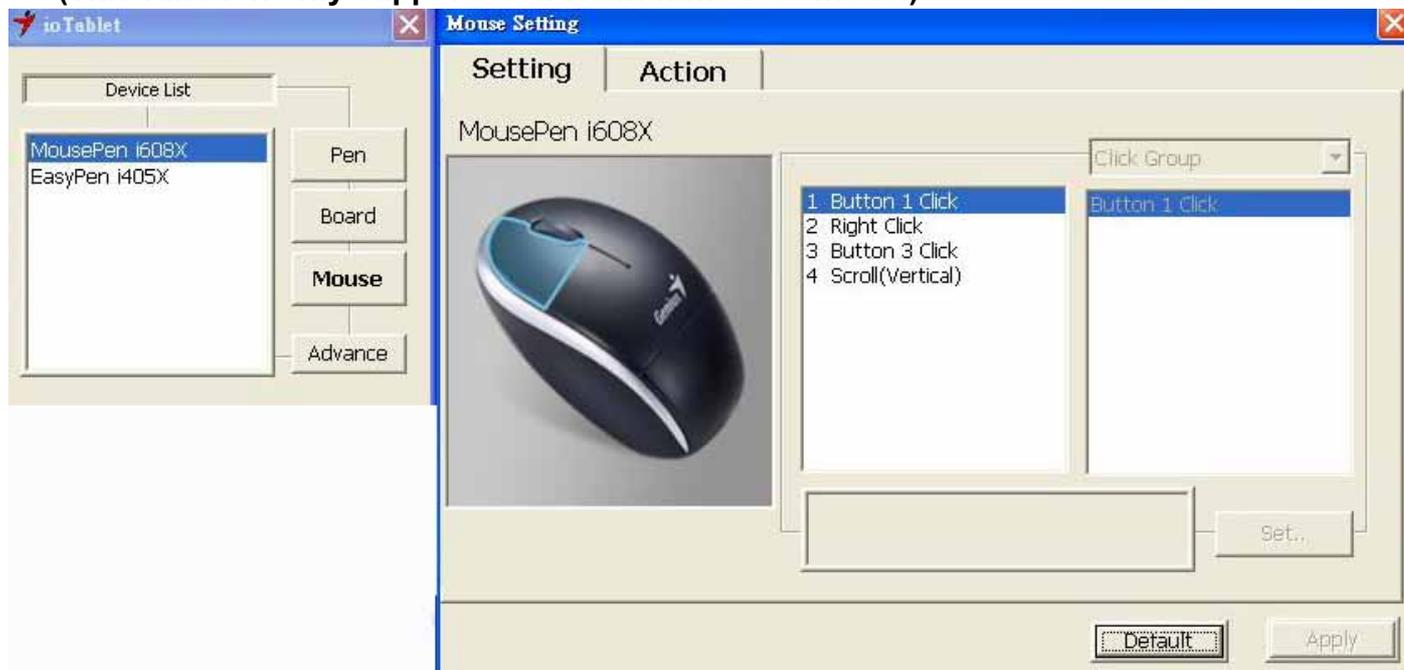
All the programmable mouse buttons are shown on the left side of the menu. Click on any of them to find out the location and the programmable setting. You may re-program any button from the drop down menu below the tablet picture.
