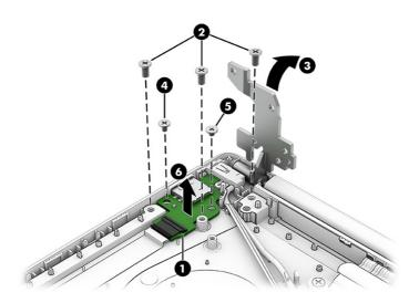
To install the USB board, reverse this procedure.
