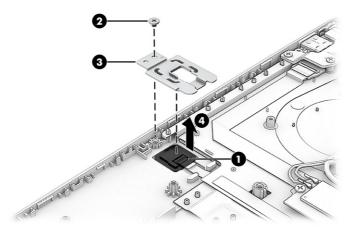
To install the fingerprint reader, reverse this procedure.
