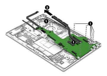
To install the system board, reverse this procedure.
