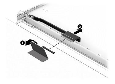
f. When replacing the display panel, use the following illustration to determine the proper installation locations of the stretchable tape on the display back cover.
