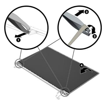
d. Remove the tape from on top of the connector on the back of the display panel (1).
