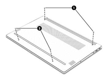
4. Insert a thin, plastic tool in the seam at the top between the bottom cover and computer to release the bottom cover, and then remove the bottom cover from the computer.
