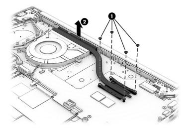
2. Thoroughly clean the thermal material from the surfaces of the heat sink and the system board components each time the heat sink is removed. Replacement thermal material is included with the heat sink and system board spare part kits. The following illustration shows the replacement thermal material location.
