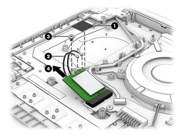
4. If the WLAN antenna is not connected to the terminal on the WLAN module, install a protective sleeve on the antenna connector, as shown in the following illustration.
