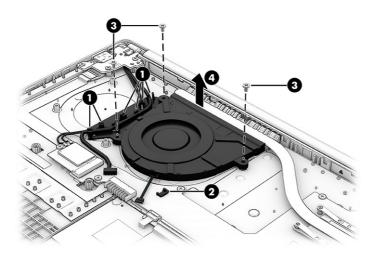
To install the fan, reverse this procedure.
