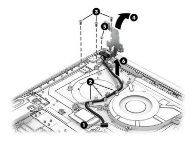
To install the power connector cable, reverse this procedure.
