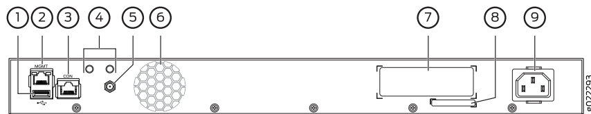
Figure 11: Rear Panel of an AC-Powered EX2300 Switch with 48 Gigabit Ethernet Ports without PoE Capability
