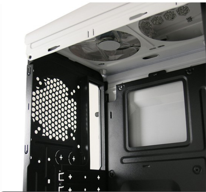
- Including two 120 mm case fans (blue lighted; 1x front; 1x top)
