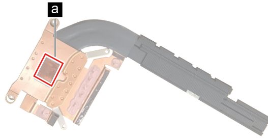
Figure 17. Areas on the heat sink where thermal interface materials should be applied (for Intel models)
