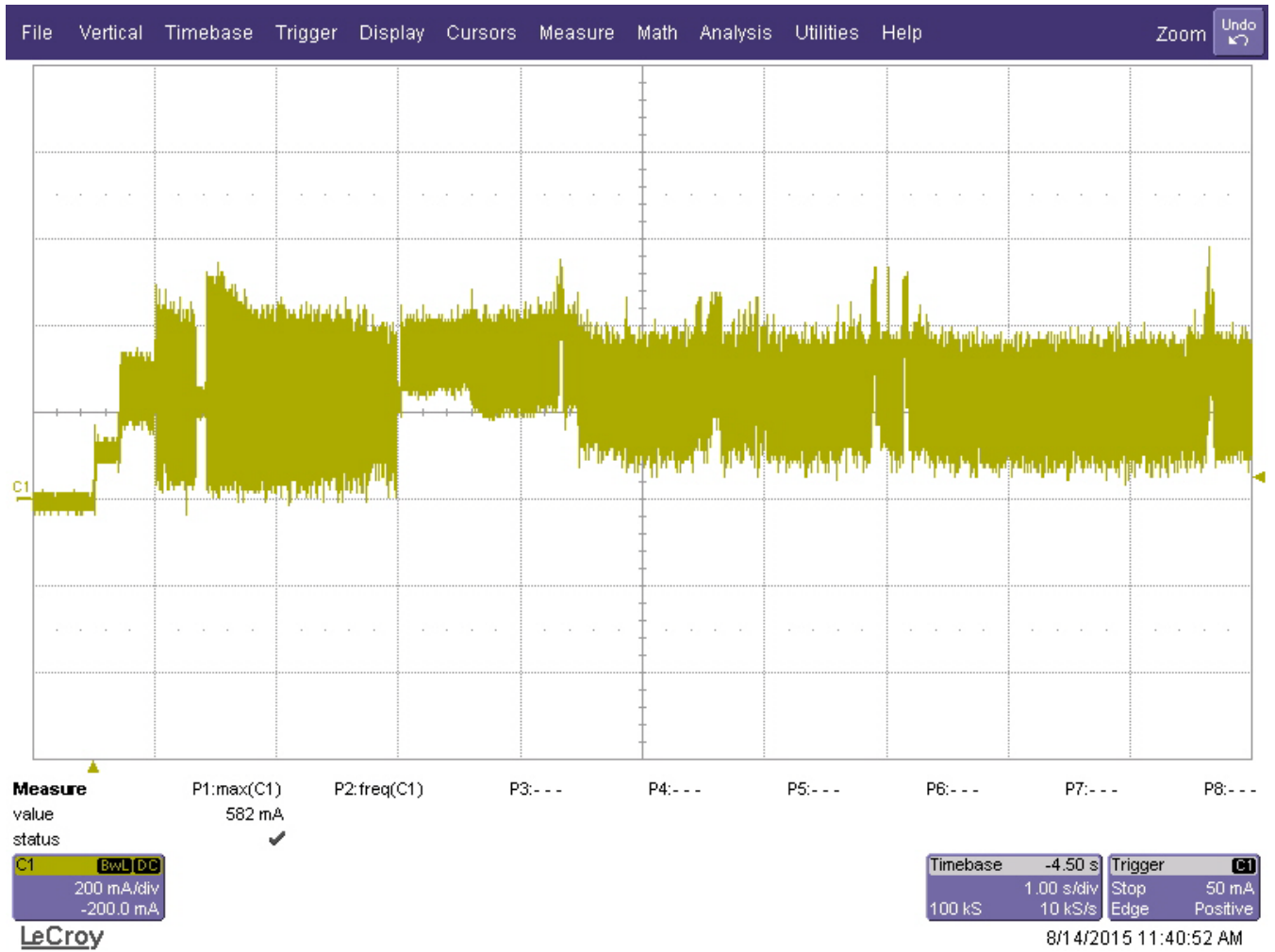
Figure 2 Typical Current Profiles (5V)
