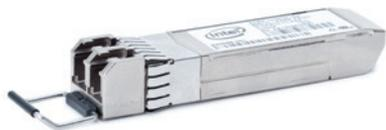
Depending on when you purchased your SFP GBIC module, it may have any of three different release mechanisms: a plastic tab on the bottom of the mini-GBIC, a wire bail, or a plastic collar around the mini-GBIC.
