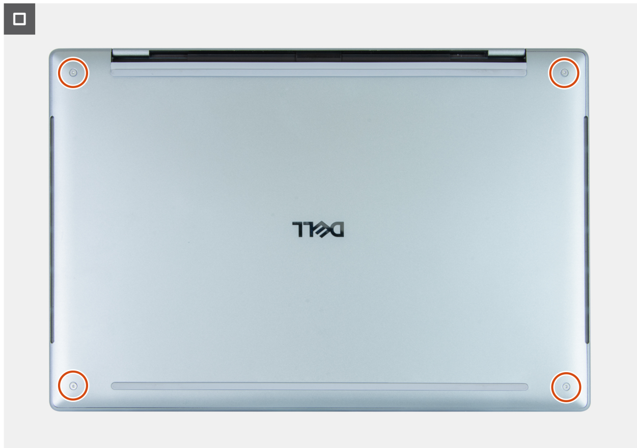
Figure 6. Replacing the screws of the base cover
