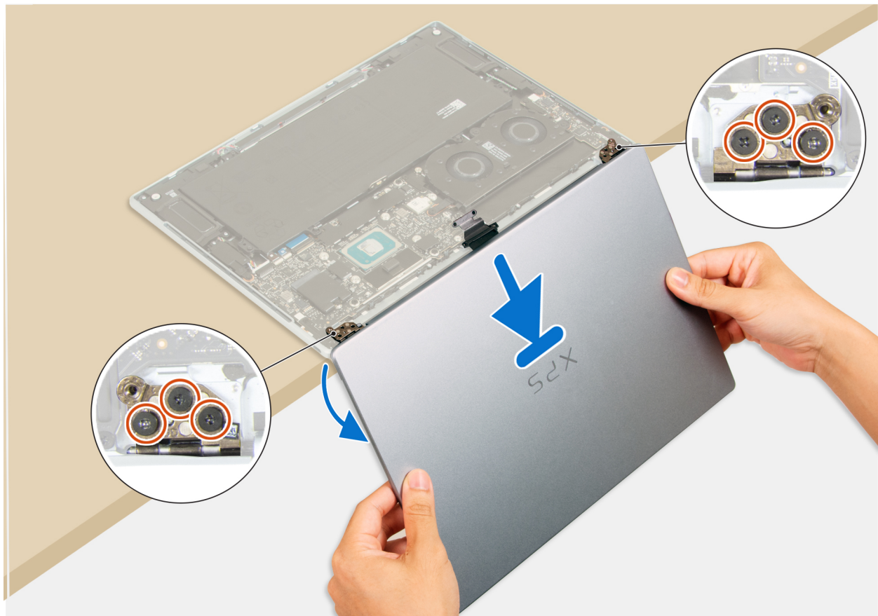
Figure 27. Removing the display assembly
