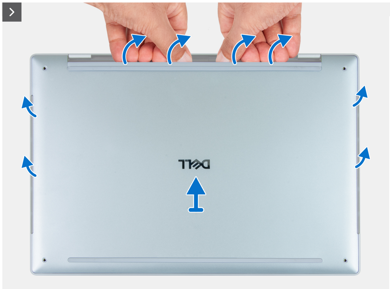
Figure 2. Opening the base cover
